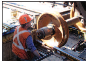
...the same table is used to raise the new wheel set into place to be installed.
