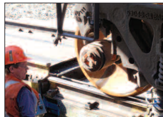
Using a specially built hydraulic table to dismount a wheel set...
